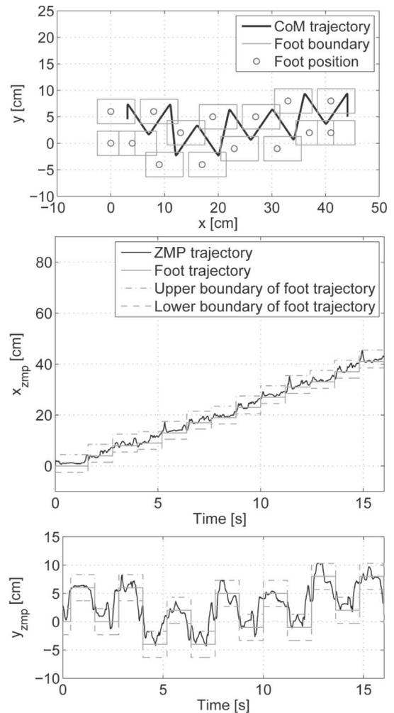
Fig. 6. Generated walking pattern, CoM, and ZMP trajectories when the plane was inclined upward and left side simultaneously in the experiment ( $\phi = 8.0^\circ$  and  $\psi = 4.0^\circ$ ).
