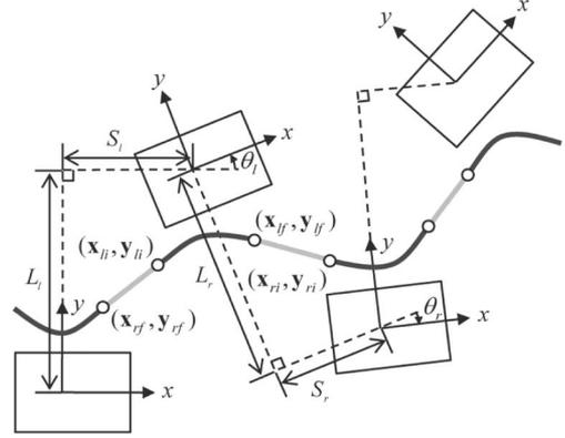
Fig. 3. Walking configuration in steady state. The rectangles represent the foot boundaries and the thick and thin lines represent the CoM trajectories in single support phase and double support phase, respectively. The small circles represent the initial/final CoM positions for left/right support phase.
