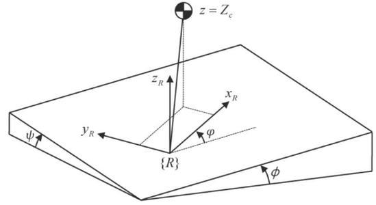
Fig. 1. 3D-LIPM on inclined plane in pitch and roll directions.
