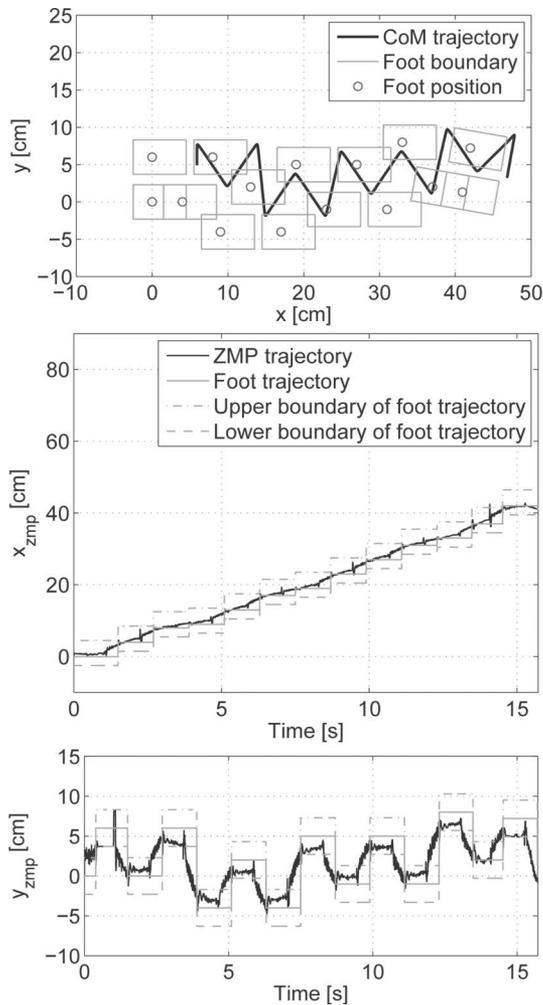
Fig. 5. Generated walking pattern, CoM, and ZMP trajectories when the plane was inclined upward and left side simultaneously in the simulation ( $\phi = 15.0^\circ$  and  $\psi = 5.0^\circ$ ).
