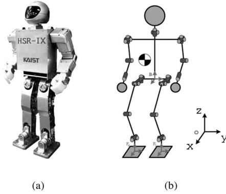
Fig. 4. Humanoid robot. (a) HanSaRam-IX. (b) Configuration.
