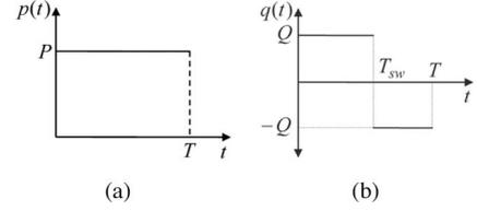
Fig. 2. ZMP functions. (a) Constant function for sagittal motion. (b) Step function for lateral motion.
