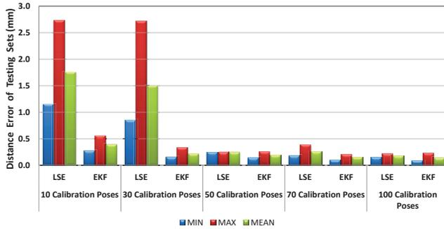
Fig. 4. Accuracy of the MyBot arm after calibration.
