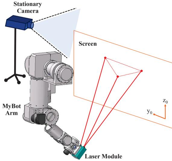
Fig. 1. Proposed kinematic calibration system.
