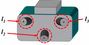
Fig. 3. Laser module having three laser sources ( $l_1$ ,  $l_2$ , and  $l_3$ ).
