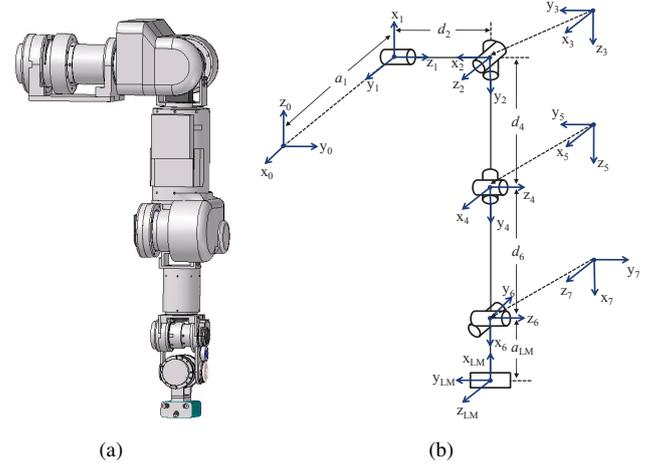
Fig. 2. MyBot arm. (a) Snapshot of MyBot arm having laser module. (b) D-H parameters and frame assignments of MyBot arm.
