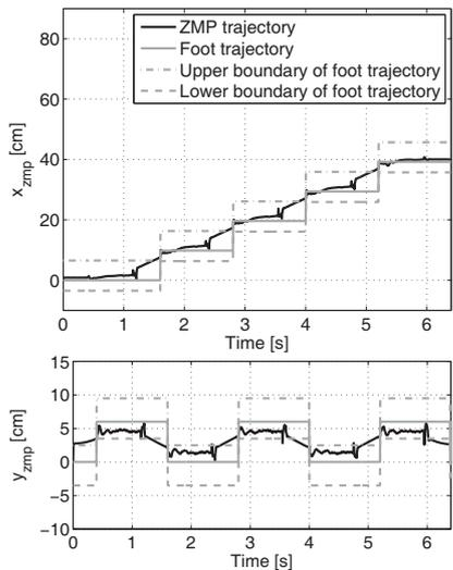
Fig. 5. Measured ZMP trajectories while walking using the COM height trajectory generated by the evolutionary optimized CPG.
