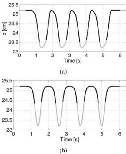
Fig. 4. COM height trajectory generated by (a) the evolutionary optimized CPG and (b) the sinusoidal function. The thick and thin lines represent the COM trajectories in the single and double support phases, respectively.
