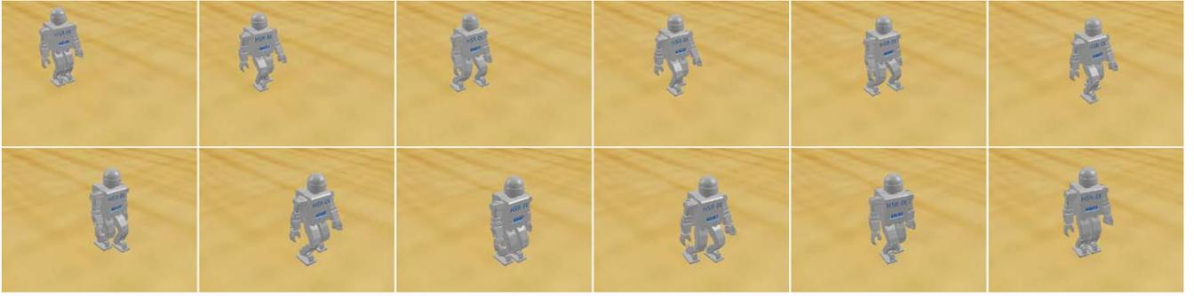
Fig. 8. Snapshots of the simulation result of modification of walking patterns while walking using the COM height trajectory generated by the evolutionary optimized CPG (left to right, top to bottom).
