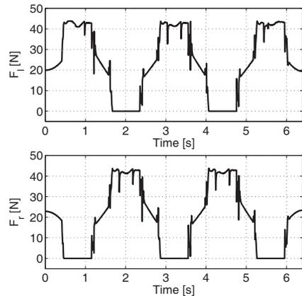
Fig. 7. Left and right GRFs while walking using the COM height trajectory generated by the evolutionary optimized CPG.
