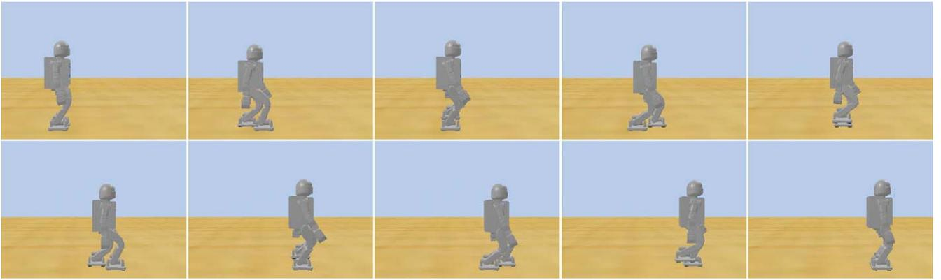
Fig. 3. Snapshots of the simulation result of straight walking using the COM height trajectory generated by the evolutionary optimized CPG (left to right, top to bottom).
