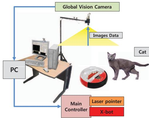
Fig. 4. Conceptual design of pet care robot system.
