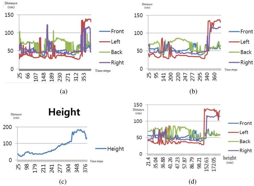
**Fig. 7** (a) Distance of horizontal ultrasonic sensors depend on time. (b) Distance of horizontal ultrasonic sensors on time (filtered). (c) Height on time (Filtered). (d) Distance of horizontal ultrasonic sensors depend on height.
