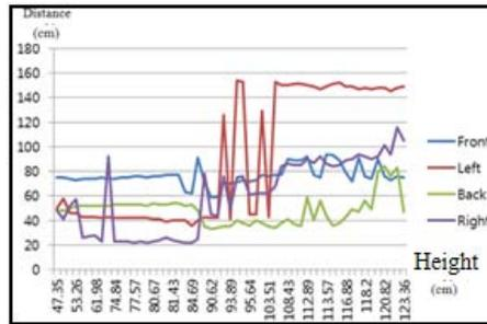
Fig. 6 Distance of horizontal ultrasonic sensors depend on height.
