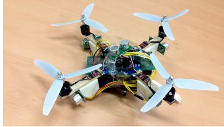
**Fig. 4** Quadcopter with sensors.
