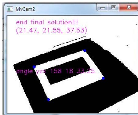
**Fig. 2** Location of camera from marker.
