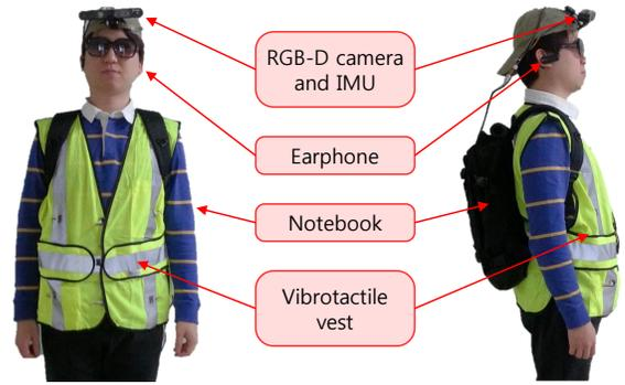
Fig. 1. The proposed an RGB-D camera-based navigational assistance system for visually impaired people
