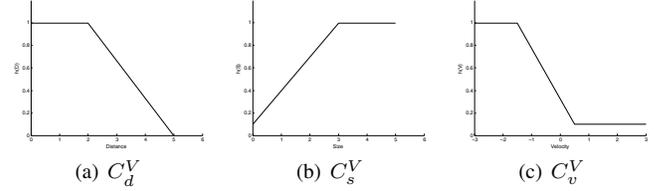
Fig. 4. Partial evaluation function for imminent-obstacle selection criteria
