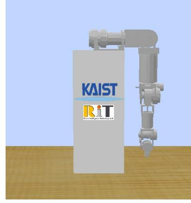
Fig. 2. Simulation model of MyBot arm in Webots simulator.
