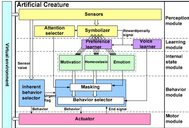
Fig. 1 Internal architecture of artificial creature, Rity
