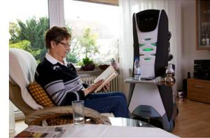
Fig. 1. Example of homecare mobile robot: Care-O-bot.
