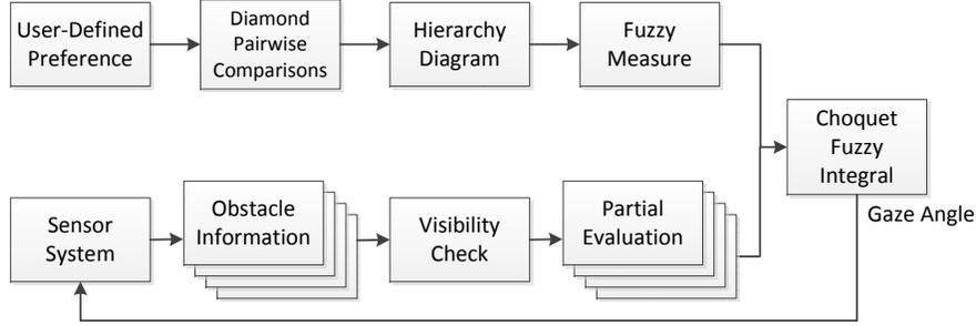
Fig. 2 Fuzzy integral-based gaze control for obstacle detection
