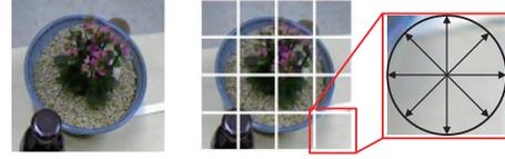
Fig. 3. A SIFT descriptor: spatial histogram of the image gradient.
