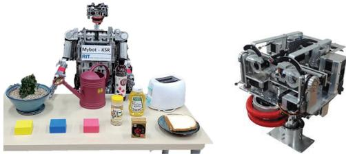
Fig. 5. Experimental setup: an RGB-D camera is mounted on the humanoid robot and all objects are on the tables.
