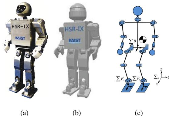
**Fig. 3.** (a) HSR-IX. (b) Simulation model. (c) Configuration.
