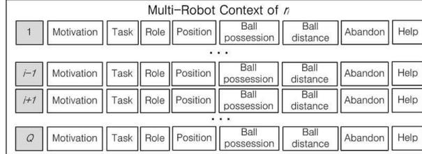
Fig. 1. Multi-robot context module.
