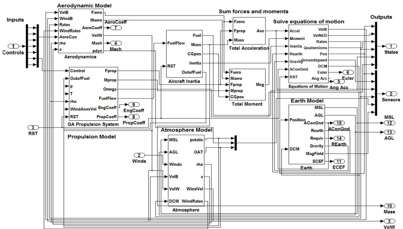
Fig. 3. The block diagram of Simulink based airplane model.
