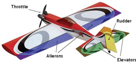
Fig. 2. Basic airplane controls.
